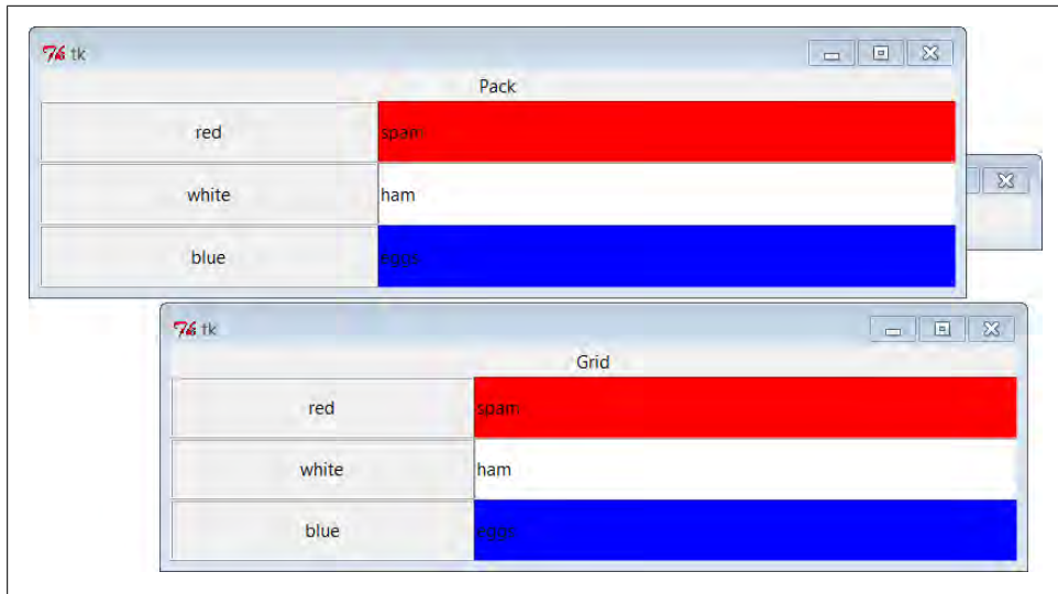
Figure 9-33. grid and pack windows resized
