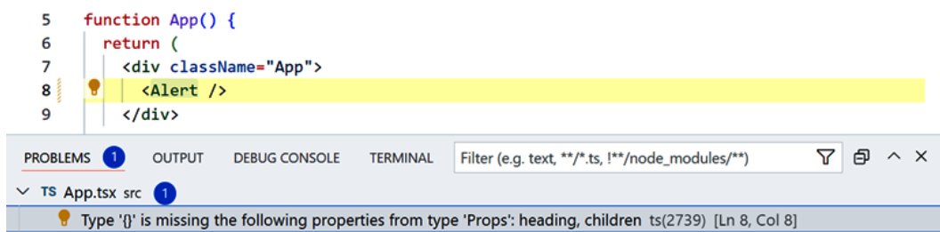
Figure 3.11 – Type error on the Alert component
